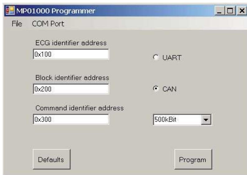
Please note that programming is only possible if pin 5 and pin 6 of X4 are shorted during power up. This is mainly to avoid unintended reprogramming of the parameters during normal operation.
